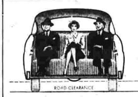
IN HUDSON, the recessed floor ("step-down" design) brings space between frame members, which is wasted in other cars, into the passenger compartment. This results in America's LOWEST center of gravity (and full road clearance), while providing more head room and seating room than any other car.
